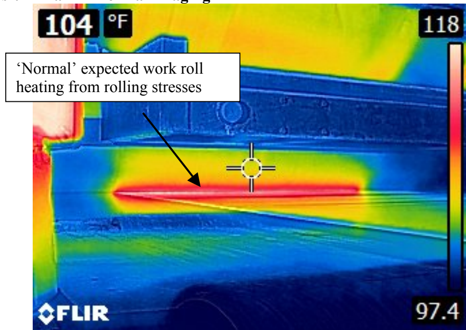
Figure 12. Successful Trial – Thermal Imaging while running
